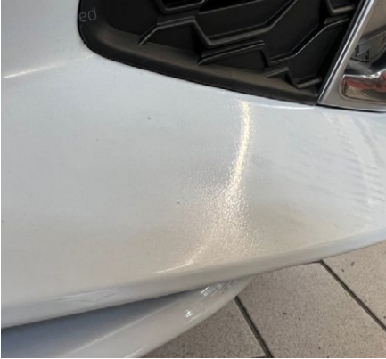
Mangelhafte Lackreparatur (Spotrepair)
